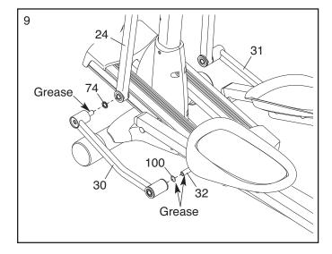
Attach the Left Link Arm (30) to the Left Pedal Arm (32) with an M8 x 15mm Button Screw (106), an M8.5 x 16mm x 1.5mm Washer (103), and an Axle Cover (66).
