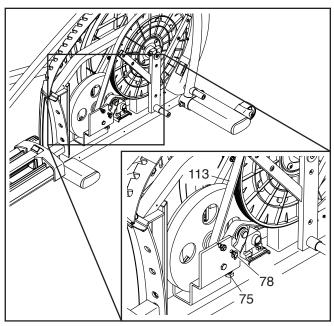
Locate and loosen the Pivot Screw (78). Next, tighten the Adjustment Screw (75) until the Drive Belt (113) is tight. Then, retighten the Pivot Screw.
