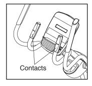
rate, hold the handgrip heart rate monitor with your palms resting against the contacts. **Avoid moving your hands or gripping the contacts tightly.**
