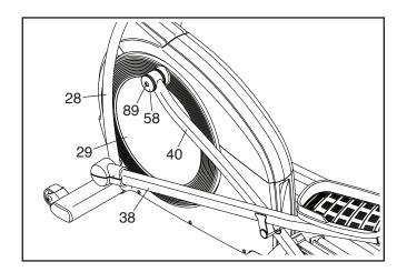
See assembly step 10 on page 11. Remove the Upper Body Covers A and B (31, 32) from the Left Upper Body Arm (27).
