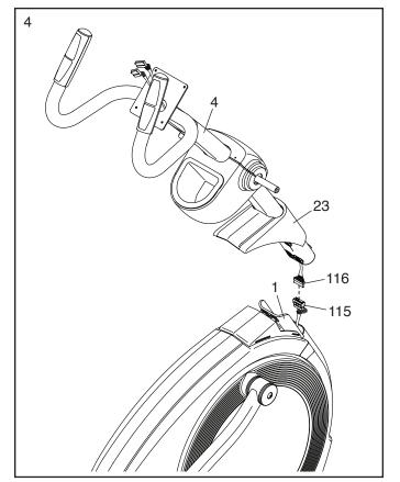
5. **Tip: Avoid pinching the wires.** Have a second person hold the Upright (4) against the Frame (1).
