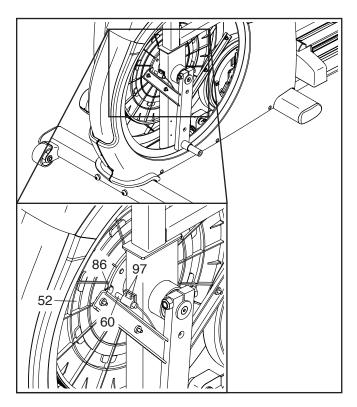
Loosen, but do not remove, the two indicated M4 x 16mm Screws (97). Slide the Reed Switch (60) slightly closer to or away from the Magnet (86), and then retighten the Screws. Then, plug in the power adapter and rock the Pulley (52) forward and backward just enough that the Magnet passes the Reed Switch repeatedly. Repeat these actions until the console displays correct feedback.
