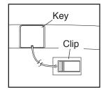
emergency, the key can be pulled from the console, causing the walking belt to slow to a stop. Test the clip by carefully taking a few steps backward; if the key is not pulled from the console, adjust the position of the clip.
