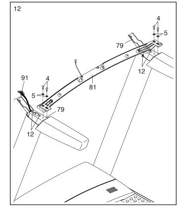
13. With the help of a second person, hold the console assembly near the Handrails (79) (only one is shown).
