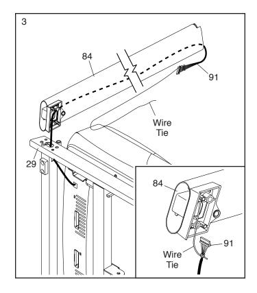
4. With the help of a second person, hold the Left Upright (84) against the Base (29). Be careful not to pinch the wires. Partially tighten three 3/8" x 4" Screws (3) with three 3/8" Star Washers (10) into the Left Upright and the Base; do not fully tighten the Screws yet.
