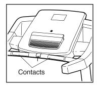
To measure your heart rate, stand on the foot rails and hold the pulse bar with your palms on the metal contacts for approximately ten seconds; avoid moving your hands. When your pulse is detected, a heart symbol in the calorie display will flash each time your heart beats, one or two dashes will appear, and then your heart rate will be shown. For the most accurate heart rate reading, continue to hold the contacts for about 15 seconds.
