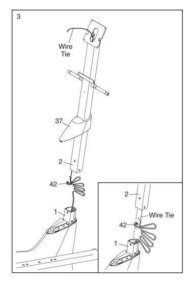
4. Slide the Upright (2) onto the Frame (1). **Tip:** Have a second person hold the Top Shield Cover (37) out of the way.
