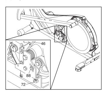
When the Drive Belt (46) is tight, tighten the Pivot Screw (88).
