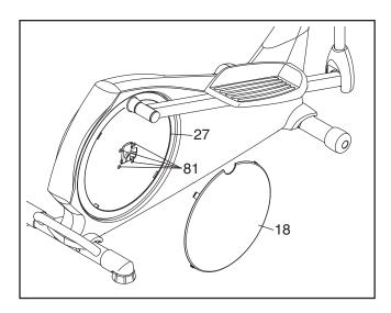
Then, remove the M8 x 14mm Button Screws (81) from the Right Pedal Disc (27), and gently rotate the Right Pedal Disc out of the way.
