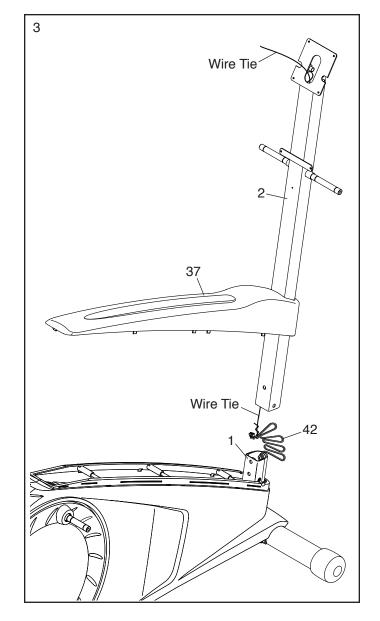
4. **Tip: Avoid pinching the Main Wire (42).** Slide the Upright (2) onto the Frame (1).
