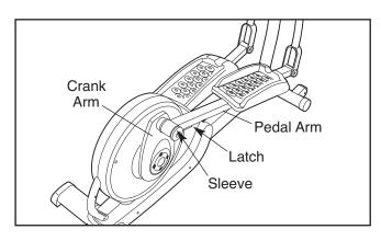
Next, raise the pedal arms until they touch the magnets on the upper body arms; the magnets will hold the pedal arms in place. Then, hold the handle and lift the frame until it locks in a vertical position.
