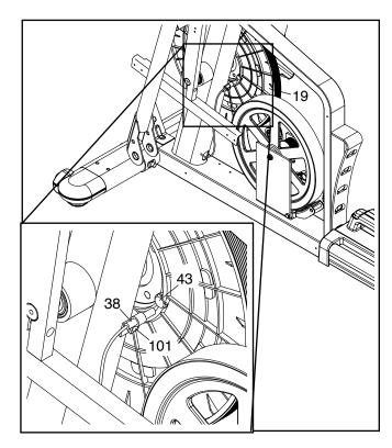
Loosen, but do not remove, the indicated M4 x 16mm Screw (101). Slide the Reed Switch (38) slightly closer to or away from the Magnet (43), and then retighten the Screw. Then, rock the Pulley (19) forward and backward just enough that the Magnet passes the Reed Switch repeatedly.
