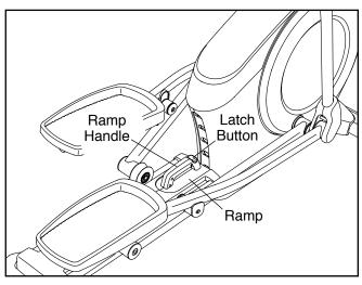
To lower the ramp, press the latch button, pull the ramp handle, and lower the ramp to the desired incline level. Then, release the latch button and engage the latch pin into one of the adjustment holes in the frame. Make sure that the latch pin is firmly engaged in one of the adjustment holes in the frame.
