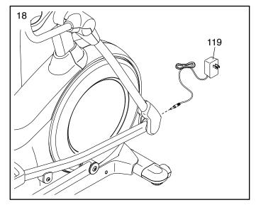
19. Make sure that all parts are properly tightened before you use the elliptical. Note: After assembly is completed, extra parts may be left over. Place a mat beneath the elliptical to protect the floor.
