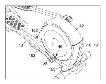
Next, lift the Latch (50) on the underside of the Left Pedal Arm (13), and then lift the Left Pedal Arm off the left Pedal Arm Sleeve (46).
