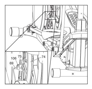
Next, loosen, but do not remove, the indicated M4 x 16mm Screw (106). Slide the Reed Switch (69) slightly toward or away from the Pulley Magnet (75). Then, retighten the M4 x 16mm Screw.
