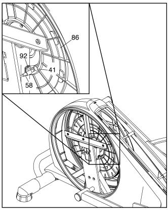
Next, rotate the Pulley (86) until a Magnet (41) is aligned with the Reed Switch (58). Slide the Reed Switch slightly toward or away from the Magnet. Then, retighten the M4 x 16mm Screw (92).
