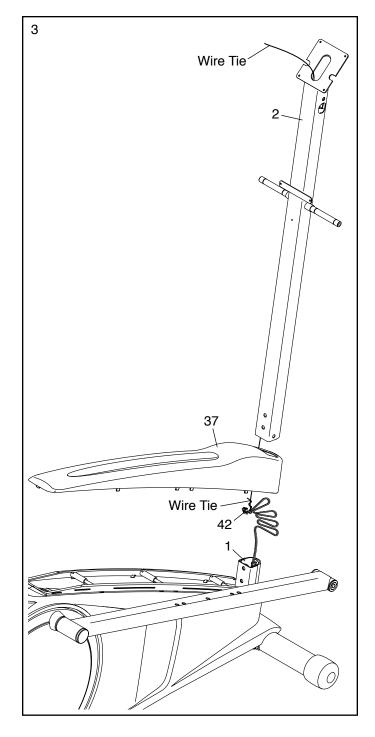
4. **Tip: Avoid pinching the Main Wire (42).** Slide the Upright (2) onto the Frame (1).
