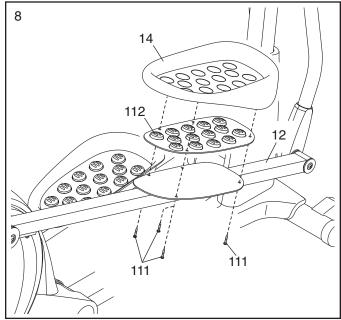
Identify the Right Upper Body Arm (8), which is marked with a "Right" sticker, and orient it as shown.
