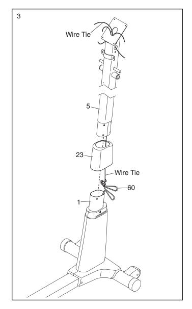
4. **Tip: Avoid pinching the Wire Harness (60).** Insert the Upright (5) into the Frame (1).
