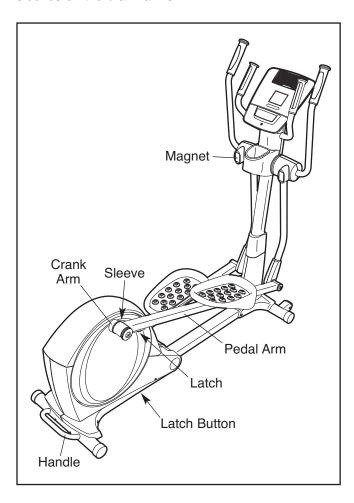
Next, raise the pedal arms until they touch the magnets on the upper body legs; the magnets will hold the pedal arms in place. Then, hold the handle and lift the frame until it locks in a vertical position.
