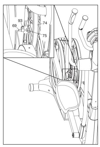
Next, rotate the Large Pulley (74) until a Magnet (75) is aligned with the Reed Switch (69). Slide the Reed Switch slightly toward or away from the Magnet. Then, retighten the M4 x 16mm Screw (93).
