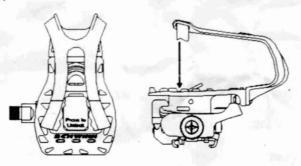
Once the locking plate has been pressed, rotate the adapter with your hands outward (away from the bike). This will take some pressure to remove it. It will help to place one hand on the front of the adapter and the other on the rear, which will maximize your leverage.
