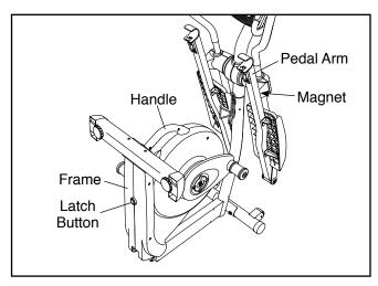
To use the elliptical, first hold the handle, press the latch button, and lower the frame.
