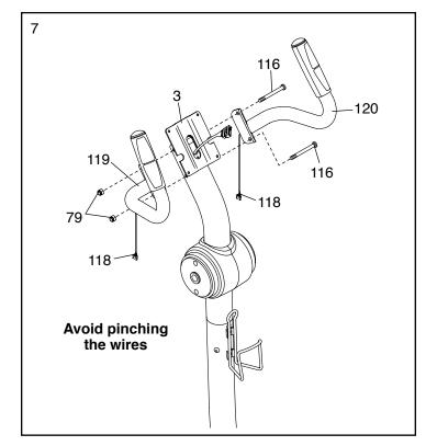
8. Insert the Pulse Wires (118) upward through the Upright (3) as shown.
