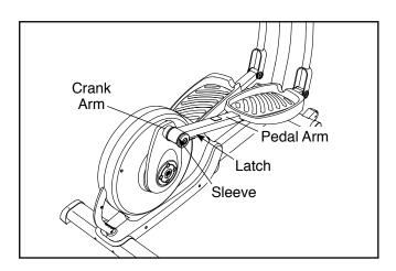
Next, raise the pedal arms until they touch the magnets on the upper body arms; the magnets will hold the pedal arms in place. Then, hold the handle and lift the frame until it locks in a vertical position.
