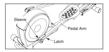
Next, raise the pedal arms until the magnets on the pedal arms touch the handlebars; the magnets will hold the pedal arms in place. Then, hold the handle and lift the frame until it locks in a vertical position.
