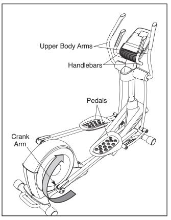
Note: The crank arms can turn in either direction. It is recommended that you turn the crank arms in the direction shown by the arrow; however, for variety you can turn the crank arms in the opposite direction.
