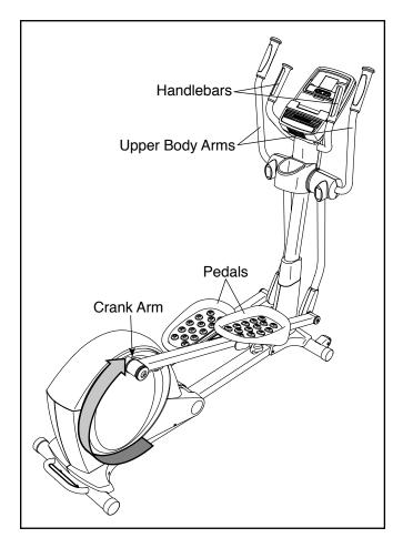
To dismount the elliptical, wait until the pedals come to a complete stop. Note: The elliptical does not have a free wheel; the pedals will continue to move until the flywheel stops. When the pedals are stationary, step off the highest pedal first. Then, step off the lowest pedal.
