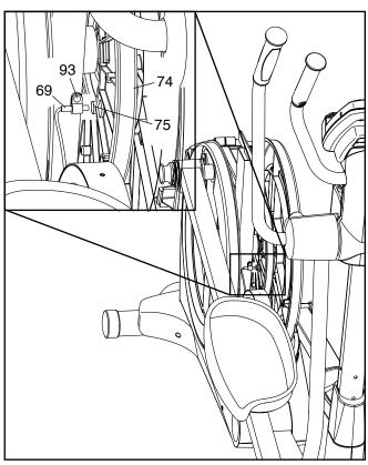
Next, rotate the Large Pulley (74) until a Magnet (75) is aligned with the Reed Switch (69). Slide the Reed Switch slightly toward or away from the Magnet. Then, retighten the M4 x 16mm Screw (93).
