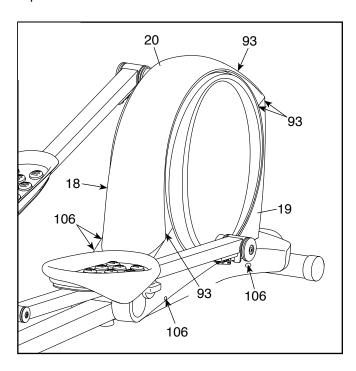
Next, remove the M4 x 16mm Screws (93) and the M4 x 42mm Screws (106) from the Right and Left Shields (18, 19). **Make sure to note which size of Screw you remove from each hole.** Then, gently remove the Left Shield.
