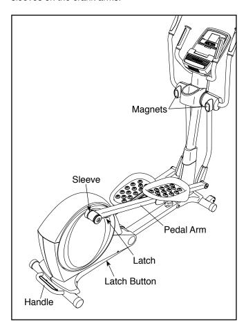
Next, raise the pedal arms until they touch the magnets on the upper body legs; the magnets will hold the pedal arms in place. Then, hold the handle and lift the frame until it locks in a vertical position. To unfold the elliptical for use, first hold the handle, press the latch button, and lower the frame.
