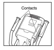
your heart rate, hold the handgrip pulse sensor with your palms resting against the metal contacts. Avoid moving your hands or gripping the contacts tightly.
