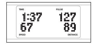
The lower left corner of the display will show your pedaling speed, in revolutions per minute.
