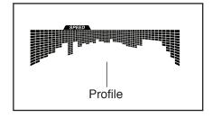
The flashing segment of the profile represents the current segment of the workout. The height of the flashing segment indicates the target speed or the incline level for the current segment.
