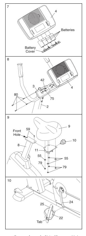
11. Make sure that all parts are properly tightened before you use the exercise cycle. Note: After assembly is completed, some extra parts may be left over. Place a mat beneath the exercise cycle to protect the floor.
