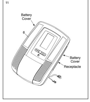
12. While a second person holds the Console (6) near the Console Plate (19), connect the wires on the Console to the Main Wire (31) and to the Pulse Wire (52).
