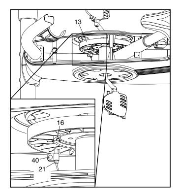
Rotate the Pulley (13) until a Pulley Magnet (16) is aligned with the Reed Switch (21). Slide the Reed Switch slightly toward or away from the Pulley Magnet. Then, retighten the M4 x 16mm Screw (40).
