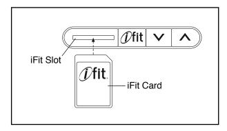
Next, select the desired workout on the iFit card by pressing the increase and decrease buttons next to the iFit slot.
