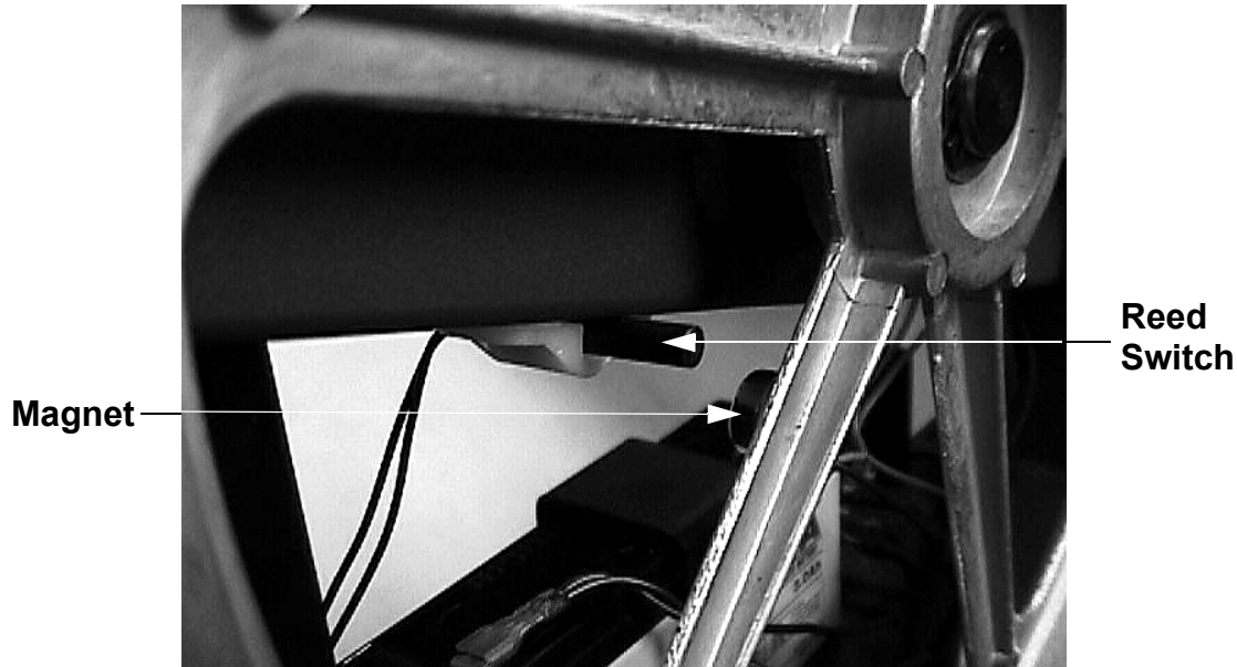
Diagram 7.14 - Speed Sensor Mounting
