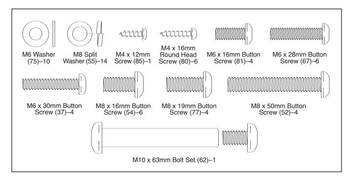
1. Orient the Left Front Stabilizer (15) with the Wheel (17) positioned as shown. Attach the Left Front Stabilizer to the left side of the Frame (1) with three M8 x 16mm Button Screws (54) and three M8 Split Washers (55).
