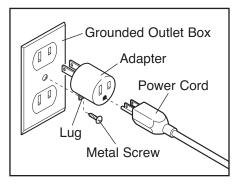
temporary adapter should be used only until a properly grounded outlet can be installed by a qualified electrician.
