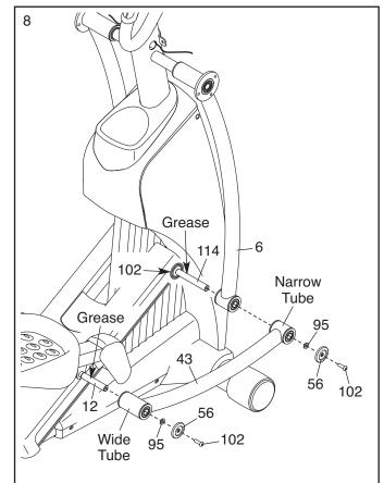
8. Identify the Right Link Arm (43), which is marked with an "R" sticker. Orient the Right Link Arm as shown.
