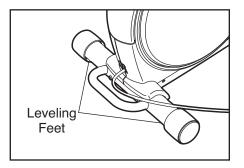
If the frame of the elliptical exerciser flexes during use, turn the center leveling foot until the flexing motion is eliminated.
