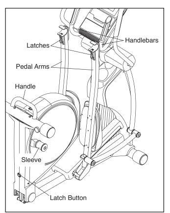
Next, raise the pedal arms until they touch the handlebars; magnets on the pedal arms will hold the pedal arms in place. Then, hold the handle and lift the frame until it locks into a vertical position.
