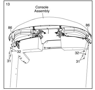
14. Set the Console (80) onto the Console Base (64). Make sure that none of the wires from the Console are pinched.
