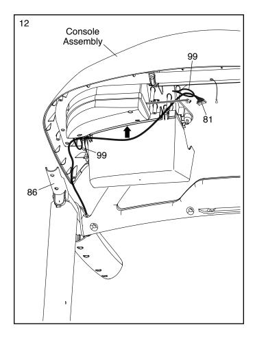
13. Set the console assembly on the brackets on the Handrails (86). **Be careful not to pinch any wires.**
