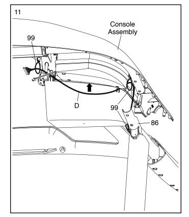
12. With the help of a second person, hold the console assembly near the right Handrail (86).
