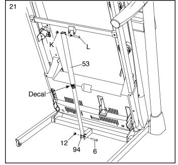
22. Attach the upper end of the Storage Latch (53) to the bracket on the Latch Crossbar (38) with a 5/16" x 2 1/4" Bolt (3) and a 5/16" Nut (12).
