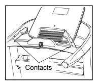
To measure your heart rate, stand on the foot rails and hold the pulse bar with your palms on the metal contacts; avoid moving your hands. When your pulse is detected, a heart symbol in the calorie display will flash each time your heart beats, one or two dashes will appear, and then your heart rate will be shown. For the most accurate heart rate reading, continue to hold the metal contacts for about 15 seconds.
