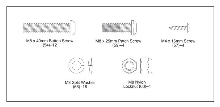
Identify the Front Stabilizer (15). While another person lifts the front of the Frame (1), attach the Front Stabilizer to the Frame with four M8 x 40mm Button Screws (54) and four M8 Split Washers (55).
