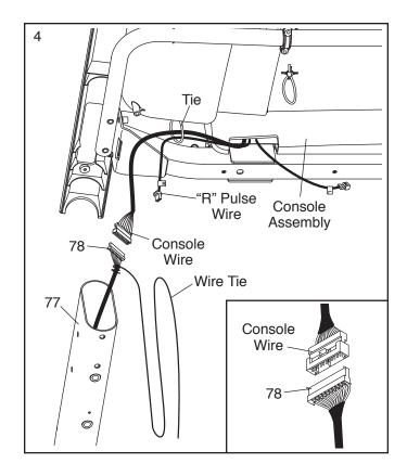
Insert the Upright Wire (78) into the right Upright (77) as you insert the Console Crossbar (101) into the Uprights. Be careful not to pinch the Upright Wire.
