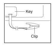
will light. IMPORTANT: In an emergency, the key can be pulled from the console, causing the walking belt to slow to a stop. Test the clip by carefully taking a few steps backward; if the key is not pulled from the console, adjust the position of the clip.
