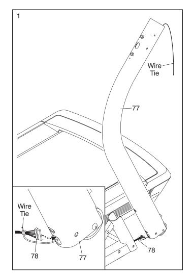
Attach the Upright (77) to the Base (80) with two 3/8" x 5 1/2" Screws (5) and a 3/8" x 2 3/4" Screw (17) with three 3/8" Star Washers (8) as shown. Start all three Screws, and then tighten them. Be careful not to pinch the Upright Wire (not shown) in the Upright.
