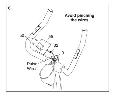
While another person holds the Console (6) near the Upright (3), connect the console wires to the Upper Wire Harness (32) and to the pulse wires.
