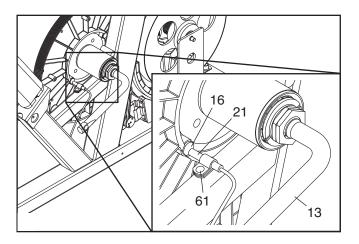
Slide the Reed Switch (21) slightly closer to or away from the Magnet (16), and then retighten the M4 x 16mm Flange Screw (61). Turn the Crank (13) for a moment.
