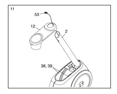
12. Orient the Console Plate (11) as shown. Then, insert the Main Wire (53) upward through the Console Plate.
