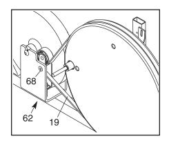
Drive Belt, you must first remove both side shields. See HOW TO ADJUST THE REED SWITCH at the left and remove the side shields.
