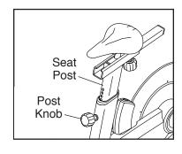
firmly tighten the post knob. Make sure that the post knob is engaged in an adjustment hole.
