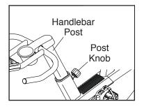
in the handlebar post, and firmly tighten the post knob. Make sure that the post knob is engaged in an adjustment hole.
