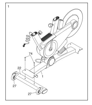
2. Attach the Rear Stabilizer (23) to the Base (1) with two 3/8" x 2 1/4" Screws (74).
