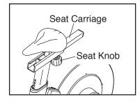
ment hole in the seat carriage, and firmly tighten the seat knob. Make sure that the seat knob is engaged in an adjustment hole.
