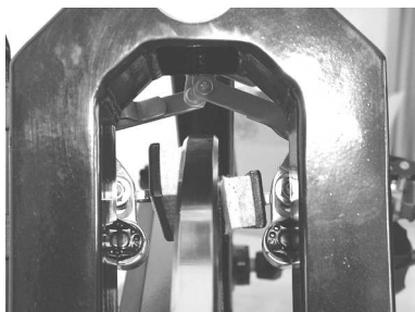
incorrect brake pad set-up
